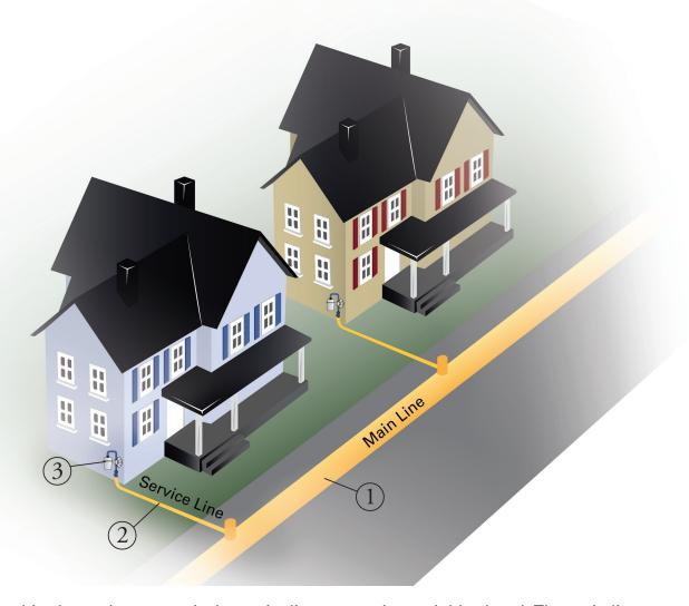
The graphic above shows a typical gas pipeline system in a neighborhood. The main line carries natural gas under the street or alley. A connection at each house or business allows gas to flow into the service line and into the building.
